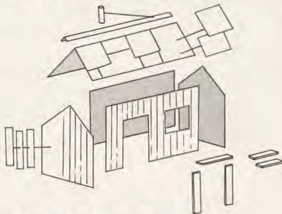
Exploded diagram of shack with tile roof
